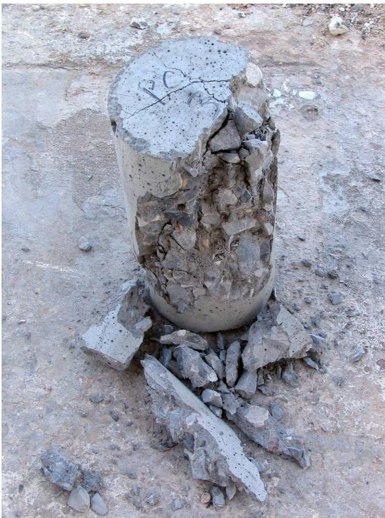
**Figure 29: Plain concrete compression failure: brittle**
