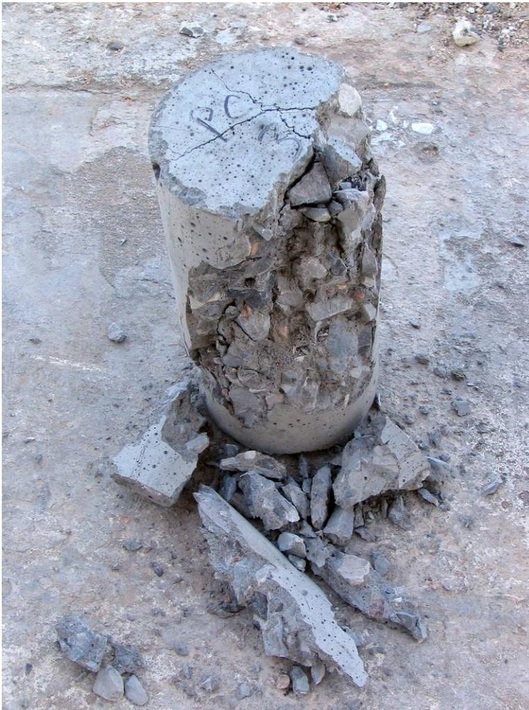
**Figure 29: Plain concrete compression failure: brittle**
