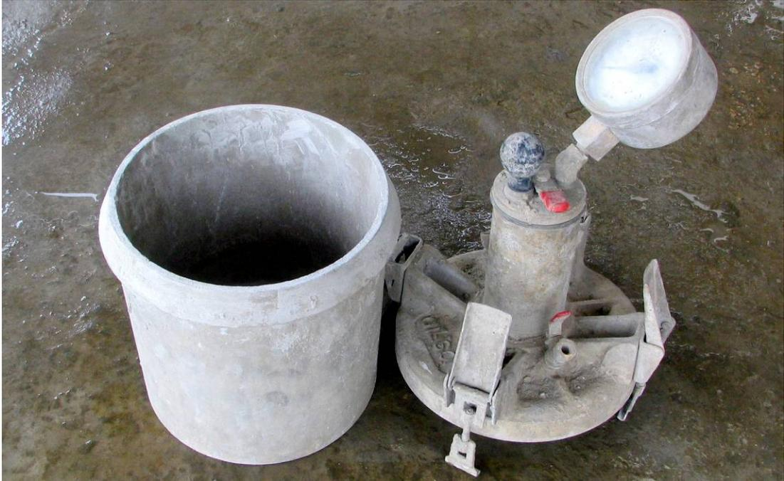
**Figure 15: Air content pressurized air pot apparatus**
