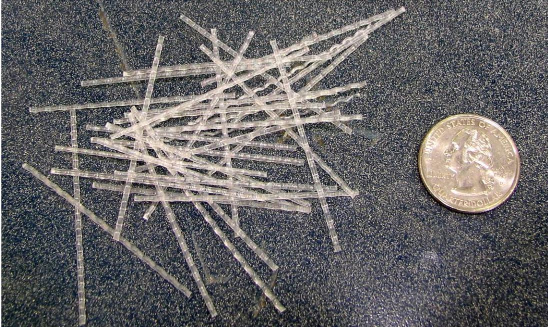
Figure 25: HPP (High Performance Polymer) fibers
