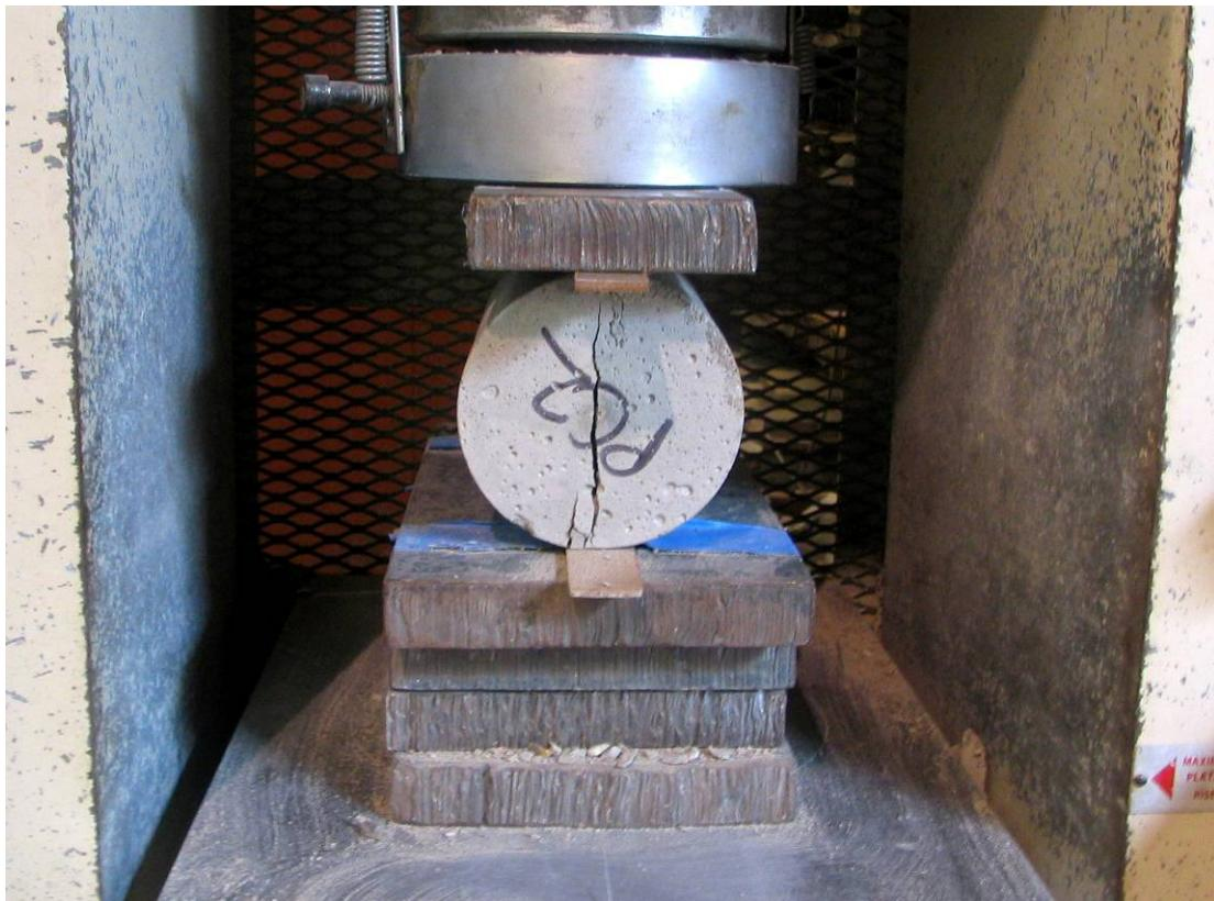
**Figure 18: Splitting tensile test**
