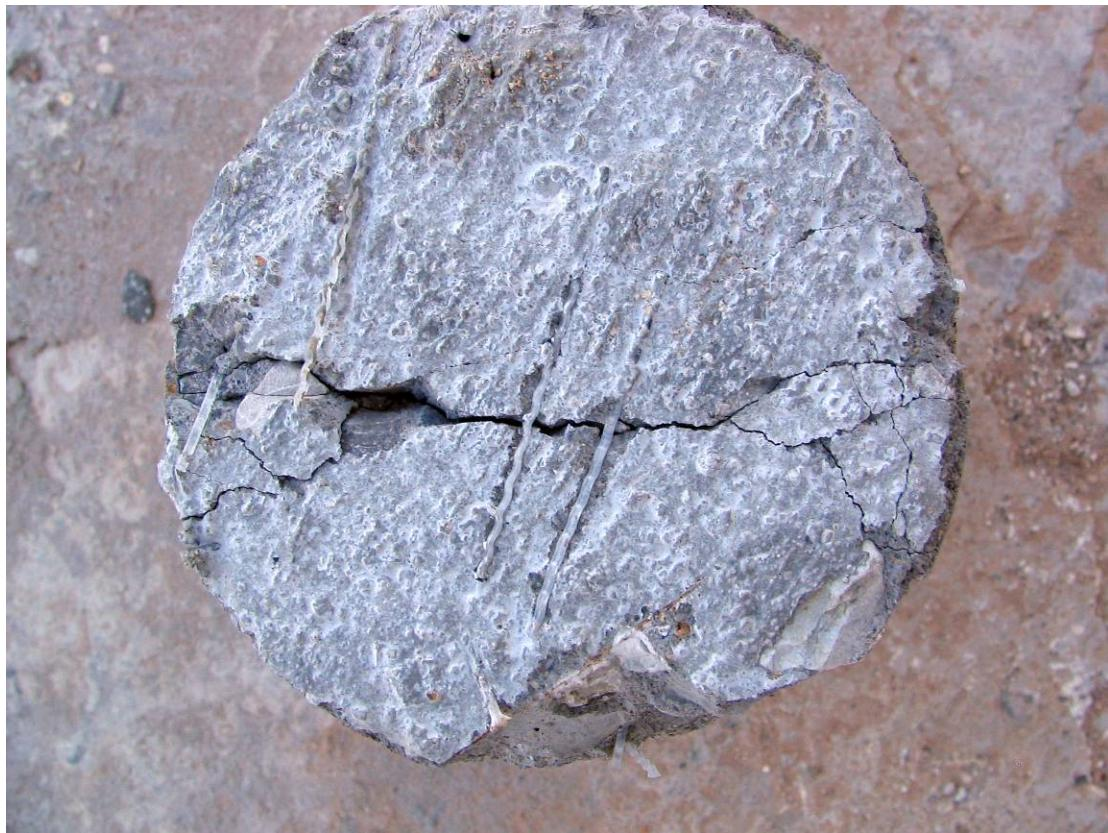
**Figure 31: Fiber-reinforced concrete splitting tensile failure: ductile**
