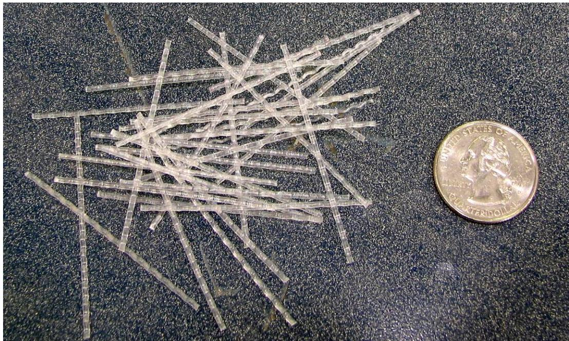
**Figure 25: HPP (High Performance Polymer) fibers**
