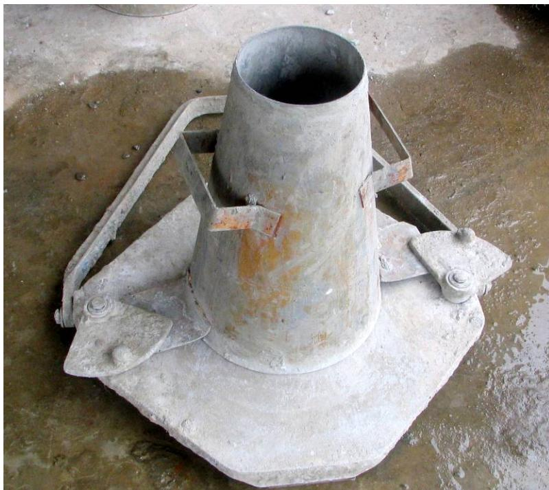
**Figure 16:** Slump test apparatus
