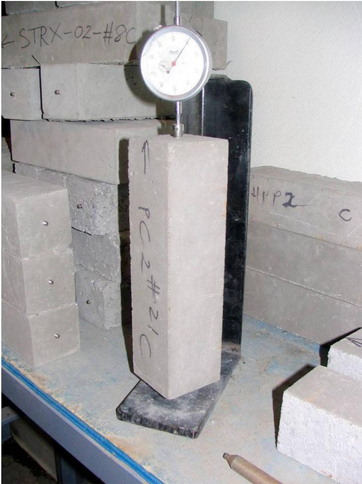
**Figure 19: Unrestrained shrinkage test**
