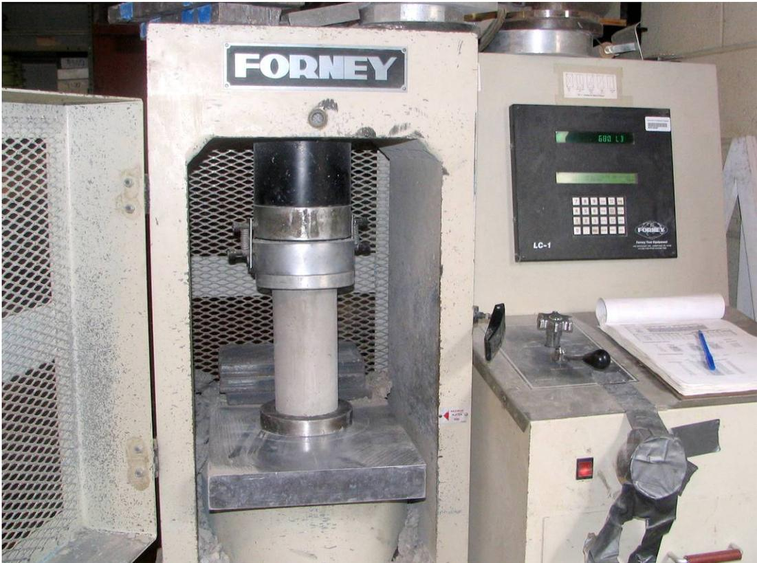
**Figure 17: Compression test with Forney compression testing machine**
