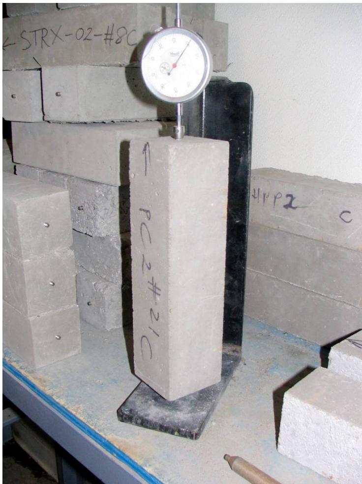
**Figure 19: Unrestrained shrinkage test**
