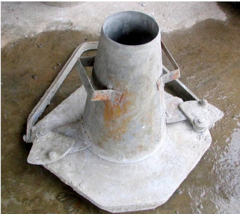
**Figure 16: Slump test apparatus**
